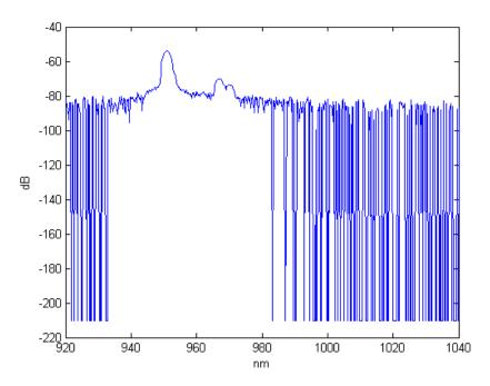
As the fiber is multimode, it seems to be hard to remove the lasing spectra and only keep the ASE using this configuration. In order to do so, we decided to change the configuration so as to couple into the fiber from the side of the laser and collect the slab modes.
