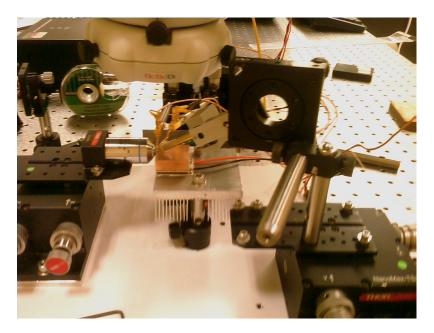
We first maximized the power coupled into the fiber through the power meter, and then looked at the spectrum on the OSA. As such, we were able to see the spectrum of the laser (back facet, with angle) as illustrated below. Because the fiber used, is a multimode fiber, the lasing emission is also coupled into the laser. We assumed that the wide spectra (920-1020nm) is the ASE.
