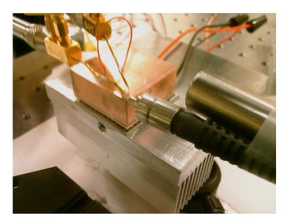
Using this configuration, however, I still saw the two peaks even from the side of the laser. The coupling improved overall, but note that this laser was the second one on the side; if one wants to test a laser farther from the side, the spectra quality can become worse than that of angle coupling.
