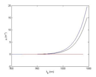
Apparently, as long as there exists a Bragg mode, the loss is lower in the lower wavelengths; hence there is not a dip in the loss calculations.
