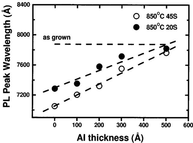
FIG. 2. Low temperature photoluminescence peak wavelength as a function of the thickness of the Al layer buried between the spin-on silica layer and the oxidized GaAs surface of an  $\text{Al}_{0.3}\text{Ga}_{0.7}\text{As}/\text{GaAs}$  QW structure. Thermal annealing was conducted at 850 °C for 20 s (solid circles) and 45 s (open circles). Dashed lines are the guides to the eyes.
