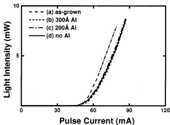
FIG. 5. Light-current characteristics for the oxide stripe lasers with band gap tuned by Al controlled QW intermixing operating at room temperature.
