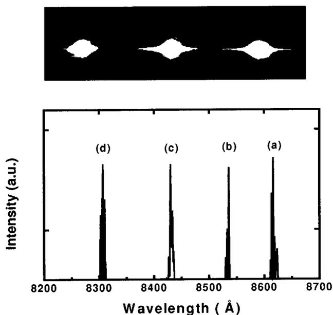
FIG. 4. Laser spectra with different blueshift by controlling the degree of quantum well intermixing with an Al layer buried between the native oxide of GaAs and the silica film. (a) As-grown laser as reference, (b) with 300 Å Al layer, (c) with 200 Å Al layer, (d) without any Al layer, and with silica on top of the oxidized GaAs surface. The RTP was conducted at 875 °C for 45 s. The upper picture is the light spot pattern at the facet of the three-wavelength laser.
