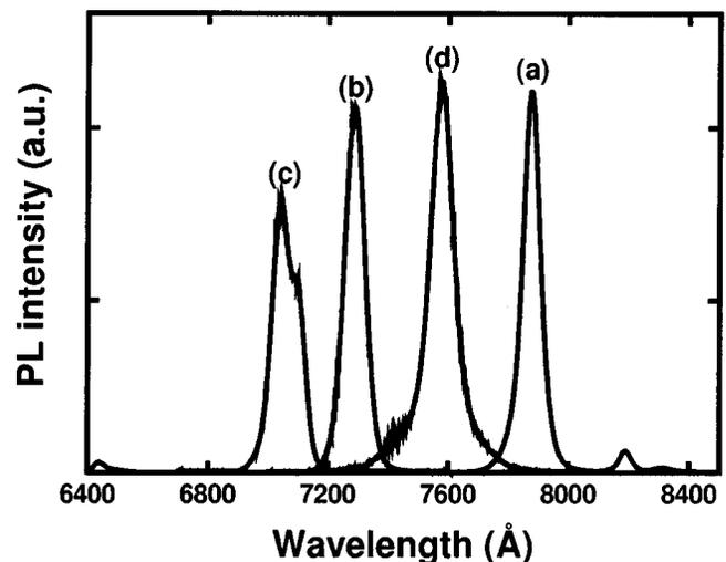
FIG. 1. Low temperature photoluminescence (7 K) spectra of Al<sub>0.3</sub>Ga<sub>0.7</sub>As/GaAs QW structures. (a) As-grown sample. (b) After 20 s of thermal annealing with a silica layer coated on an oxidized surface. (c) After 45 s of thermal annealing with a silica layer coated on an oxidized surface. (d) After 20 s of thermal annealing with a 20-nm-thick Al layer buried between a coated silica layer and an oxidized surface. The annealing temperature was 850 °C.
