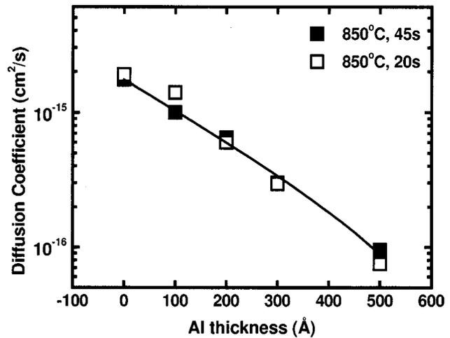
FIG. 3. Interdiffusion coefficient at 850 °C as a function of the thickness of the Al layer buried between the spin-on silica layer and the oxidized GaAs surface of  $\text{Al}_{0.3}\text{Ga}_{0.7}\text{As}/\text{GaAs}$  QW structure. Thermal annealing time was 20 s (open squares) and 45 s (solid squares). The solid line is an exponential fitting curve.
